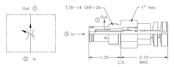
Operation Controls flow from the port 2 to port 1 at an adjusted value over a varying pressure range.
